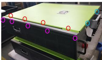
Open the top cover slowly. Before you can open it totally, please don't forget to remove the cables attach the LCD:
