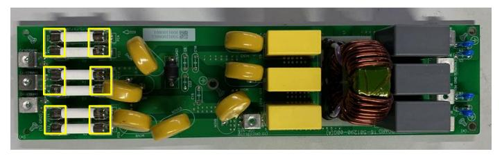
Please measure the resistance of the two side of the fuse, they should be 0ohm.
